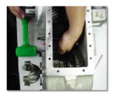
11. Remove the forks from the case. (Note: If you have Atlas case #1929 or earlier and have not upgraded your shifter forks, this is an ideal time to install new shift forks, P/N 301550).
